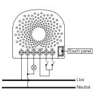
Wiring diagram of 2-Wire system.
